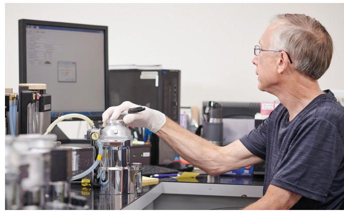
"The vaporizer needs to be serviced in a climate-controlled room," Ishmael said. "And that's very important for setting the thermostats. The thermostat actually controls the vaporizer's output. It will hold accuracy between 58 degrees Fahrenheit and 95 degrees Fahrenheit. It's very important that it's serviced in an area that's temperature and climate controlled in a room where you have service technicians who know what they're doing."
